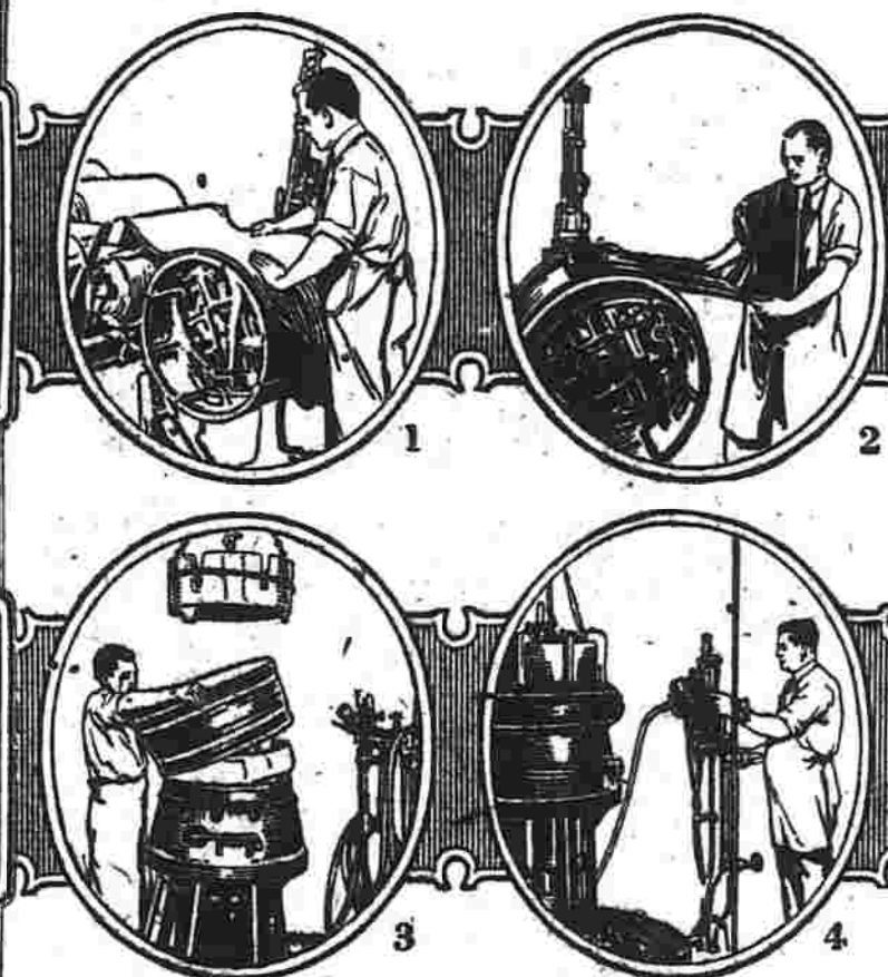
Steps in Building a United States Tire by the Flat Band Method. 1. Laying plies of Latex-treated Web Cord on drum. 2. Applying tread rubber. 3. Placing tire on inflation machine. 4. Inflation finished. Tire formed.
